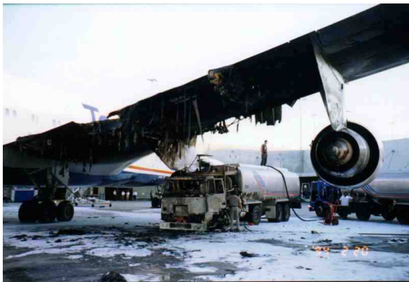
Pictures 6 and 7: Static electricity as a cause for fire on the aircraft “Towerair”
