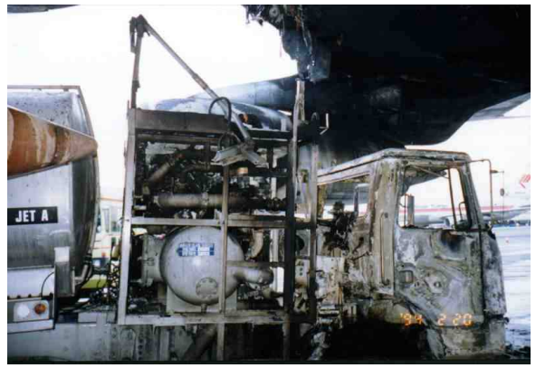
Pictures 6 and 7: Static electricity as a cause for fire on the aircraft “Towerair”
